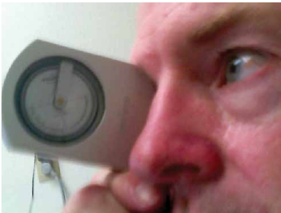
Figure 1. Using a clinometer to measure tree height. Note scale on the dial.
