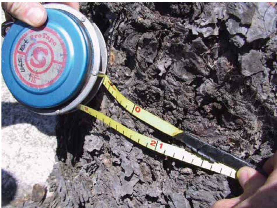
Figure 2. A diameter tape converts tree circumference to diameter in inches. This tree is 21.5 inches in diameter.
