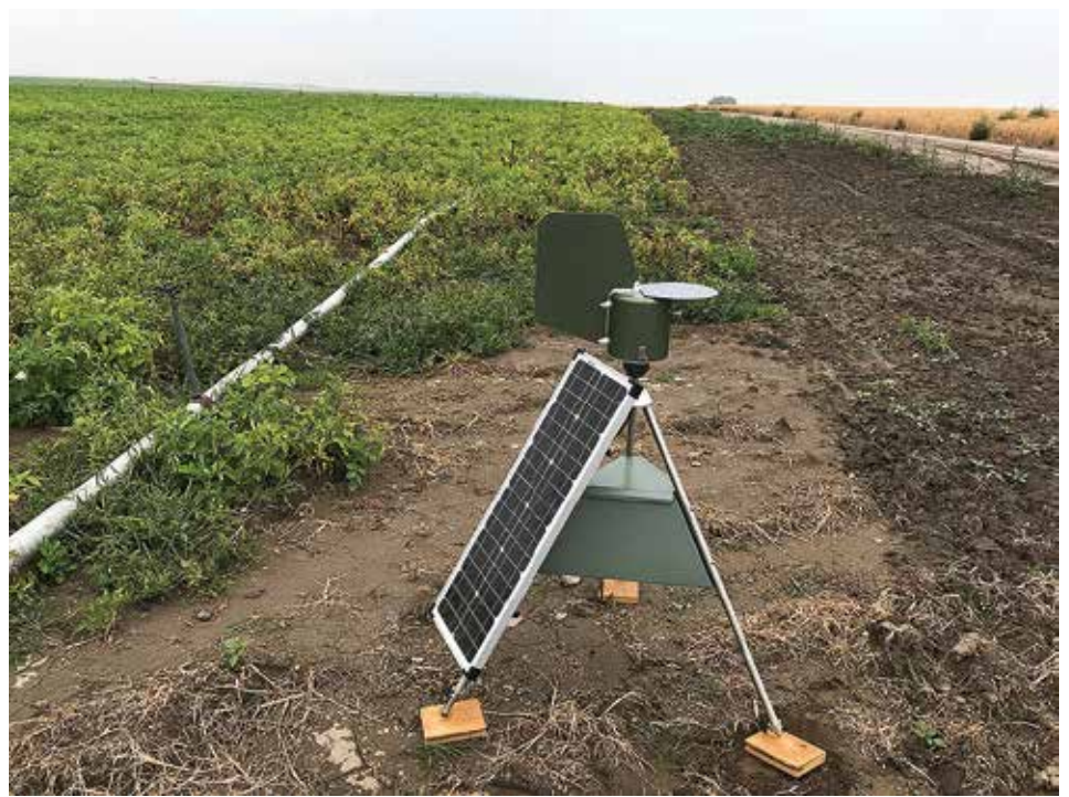
A network of spore traps, like the one shown here, have helped University of Idaho researchers keep tabs on the arrival of fungal pathogens.
