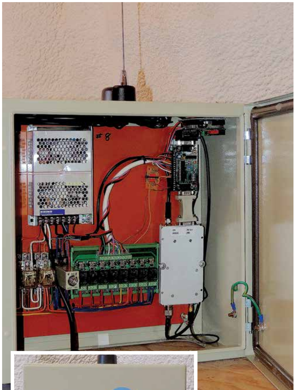
Photos by Dianna Troyer The interior of a Remote-Ag box, which Milo Call designed to remotely control his pivots using UHF radios. LEFT: RemoteAg uses a radio antenna, global positioning system, and a command board that relies on a timer and series of relay switches.
