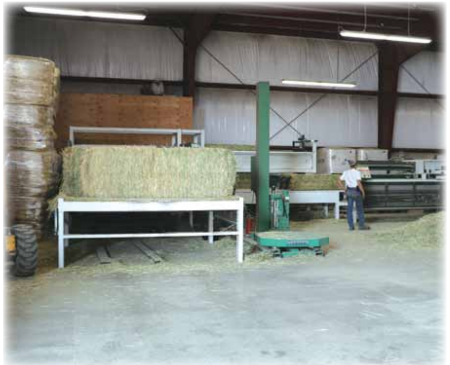
A soft press in operation near Rathdrum. The machine cuts, reties and repackages large bales into smaller bales. Photo by Steve Ritter
