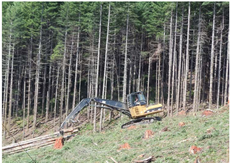
Shovel logging, using tracked loaders, is an excellent practice to reduce soil impacts.
