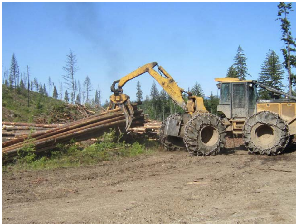
Ground-based skidding using a grapple skidder; machines can have rubber tires or tracks.
